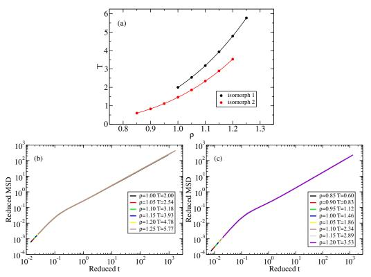
**Figure 1.** (a) The two LJ isomorphs studied. State points on the isomorphs were found by integrating Equation (4) numerically. (b) Mean-square displacement (MSD) for the state points of isomorph 1 plotted in reduced units, demonstrating good isomorph invariance of the dynamics. (c) The same for the state points of isomorph 2.
