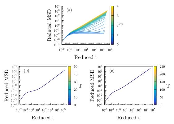
**Figure 3.** A particle mean-square displacement in reduced units of three different sets of simulations of the Wahnström binary LJ mixture [46]. (a) gives MSD data along the  $\rho=0.85$  isochore (where density is given in AA particle units). (b) is for the isomorph with reference state point  $(\rho,T)=(0.85,1.2)$ . (c) is for the isomorph with reference state point  $(\rho,T)=(0.85,2.0)$ .
