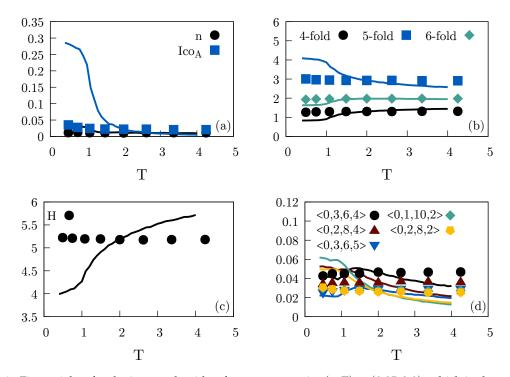
Figure 5. As in Figure 4, but for the isomorph with reference state point  $(\rho, T) = (0.85, 2.0)$ , which is above the freezing line. The isochore is given by  $\rho = 0.85$ . The structures are isomorph invariant to a good approximation, but vary along the isochore. Note that compared to Figure 4 there are more low-probability Voronoi structures, with no dominant structural motif.
