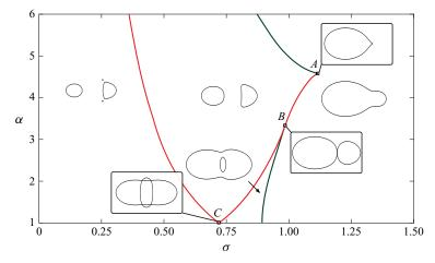
Figure 4. Bifurcation diagram of the merging process in the core growth model for  $\alpha \ge 1$ . The bifurcation curves separate the ( $\sigma$ ,  $\alpha$ ) parameter plane into four distinct regions with different vortex topologies. Crossing a green (red) part of the bifurcation curve results in a punching (pinching) bifurcation.
