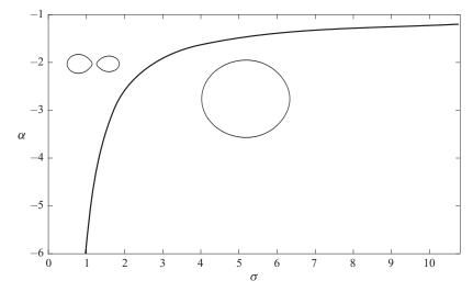
Figure 6. Bifurcation diagram of the merging process in the core growth model for  $\alpha < -1$ . The green bifurcation curve separates the  $(\sigma, \alpha)$  parameter plane into two distinct regions with different vortex topologies. The topological structures are illustrated with an example of a Q = 0 contour curve within each region. On the bifurcation curve one of the vortices disappears in a punching bifurcation.
