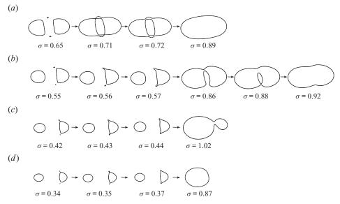
Figure 7. Navier–Stokes simulations at Re = 10. The evolution of the vortex structure is shown at selected values of  $\alpha \ge 1$ . For each value of  $\alpha$ , all the structurally stable topologies of the Q = 0 contour curve are shown in the order of evolution. (a)  $\alpha = 1$ ; (b)  $\alpha = 2$ ; (c)  $\alpha = 4$ ; (d)  $\alpha = 6$ .
