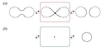
Figure 1. Illustration of the local changes in the structure of the Q = 0 contour curves during a (*a*) pinching and a (*b*) punching bifurcation. The bifurcation states are depicted in red and green boxes. The dashed lines in (*a*) show an example of a possible global structure during a pinching bifurcation. Note that the empty left panel in (*b*) illustrates that there are no Q = 0 contour curves.
