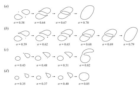
Figure 8. Navier–Stokes simulations at Re = 100. The evolution of the vortex structure is shown at selected values of  $\alpha \ge 1$ . For each value of  $\alpha$ , all the structurally stable topologies of the Q = 0 contour curve are shown in the order of evolution. (a)  $\alpha = 1$ ; (b)  $\alpha = 1.2$ ; (c)  $\alpha = 3$ ; (d)  $\alpha = 5$ .
