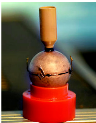
FIG. 8. The piezo-ceramic transducer used for measuring the dynamic adiabatic bulk modulus. 28–30,67,68 The device consists of a piezo-electric ceramic shell with electrodes on both sides with wires connected to a frequency analyzer. The inner diameter is 18 mm and the shell thickness is 0.5 mm. A small hole in the shell makes it possible to fill the transducer with liquid at room temperature at which the viscosity is low. A tube acting as a liquid reservoir is attached on top of the hole, which ensures that the sphere remains filled as the liquid inside contracts upon cooling.
