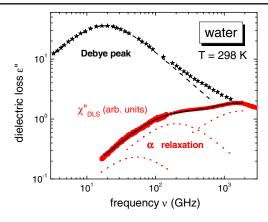
FIG. 1. Comparison of dielectric (black stars, taken from Ref. [29]) and DLS (red dots, current work) susceptibilities for water at room temperature. The dashed black line corresponds to a Debye function. The solid black line is a fit of DLS spectrum with the sum of two Debye functions, accounting for the contributions of relaxation processes, and an arbitrary peak function considered for the fast dynamics. The red dotted lines highlight the individual contributions composing the DLS spectrum.
