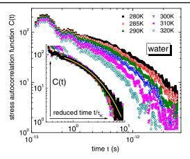
FIG. 2. Temperature evolution of stress correlation function C(t) obtained from computer simulations. The inset shows the master curve obtained by the horizontal shift of the individual C(t) data sets. The (yellow) solid line is a fit with a stretched exponential function.
