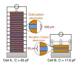
FIG. 1. Schematic drawings of the two cells used for the crystallization studies. Cell A is a multi-layer capacitor with gold plated electrodes (variable capacitor type used in old fashioned radios) with a geometric capacitance of 65 pF. Cell B is a two-plate capacitor with beryllium copper electrodes and 50  $\mu$ m sapphire spacers. Cell B has a geometric capacitance of 17.6 pF.
