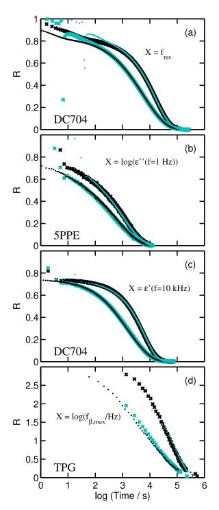
FIG. 4. Data (crosses) and predictions based on Eq. (10) (dots) for each of the normalized Fig. 2 data sets. (a) Mechanical resonance frequency; (b) low-frequency dielectric loss; (c) high-frequency dielectric constant; and (d) beta loss-peak frequency. Up jumps are in black, down jumps in light blue. The predicted curves are in the same color as the data they are calculated from.
