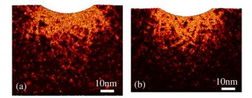
**Figure 8.** Comparison of MgCu (a) and CuZr (b) metallic glass under otherwise identical nanoindentation conditions. The latter shows the strongest shear localization.
