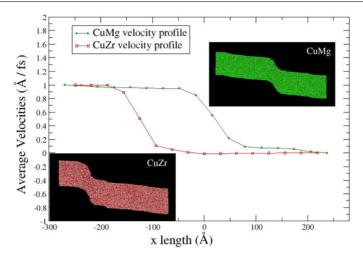
Figure 2. Shear deformation on CuZr and MgCu thin sample and the velocity profile with respect to the length. The width of the shear bands were found to be  $5-6\,\mathrm{nm}$  for CuZr and  $8\,\mathrm{nm}$  for MgCu.
