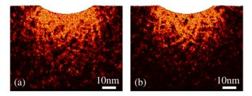
**Figure 7.** Influence of varying the cooling rate during glass formation. Samples created with cooling rates of  $2.2\,\mathrm{K\,ps^{-1}}\,(a)$  and  $0.44\,\mathrm{K\,ps^{-1}}\,(b)$  were subjected to otherwise identical nanoindentation simulations. The shear localization appears stronger in the more slowly cooled sample.
