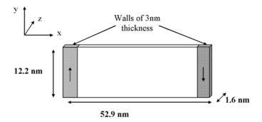
**Figure 1.** The setup used for simple shear deformations. The shear is applied by forcing the walls to move as indicated by the arrows. There are periodic boundary conditions in the y and z directions.
