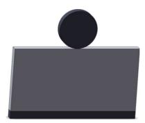
**Figure 3.** The geometry used during nanoindentation. The cylindrical indenter is modeled as a repulsive potential. There are periodic boundary conditions in the x and y directions (left-right and out of the plane of the paper). The upper surface is free, the lower surface is held fixed by fixing the positions of all atoms in a 0.8 nm thick layer.
