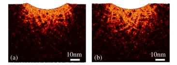
**Figure 5.** Influence of varying the indentation velocity on shear band formation and on load-displacement curves. The indentation velocities are  $30 \,\mathrm{m\,s^{-1}}$  (panel a) and  $7 \,\mathrm{m\,s^{-1}}$  (panel b). The shear bands are less developed during the fast nanoindentation. The corresponding load-displacement curves are shown in figure 4(e).
